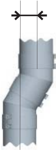
Figure 28 – MINIMUM OFFSET for ELBOWS
